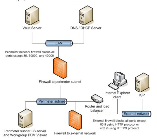
The Internet Explorer client connects to the Workgroup PDM Viewer/IIS server by way of port 80 (or 443 if configured to use SSL). The Workgroup PDM Viewer then connects to the Vault server using ports 30000 or 40000. The Vault server sends the requested information back to the Workgroup PDM Viewer, which then feeds the information back to the Internet Explorer client.
