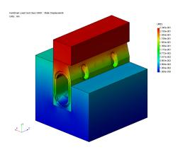
SolidWorks Simulation helped ACO designers understand exactly where the KerbDrain might fail under certain load conditions.
