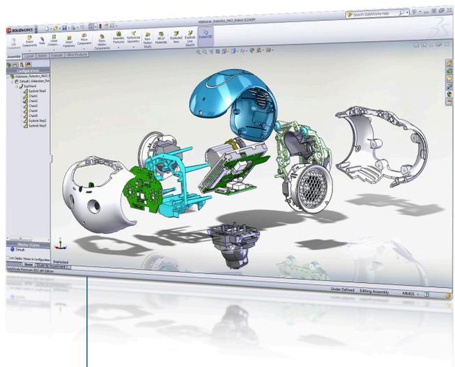
Using integrated SOLIDWORKS simulation tools, Aldebaran optimizes part performance as well as the production of injected-molded components.
