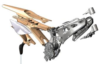
Using SOLIDWORKS Simulation tools, Alta Motors overcame technical challenges while improving motorcycle performance, such as eliminating a third of the design's mass and shaving off an additional 10 percent of its weight, resulting in increased strength and better manufacturability.
