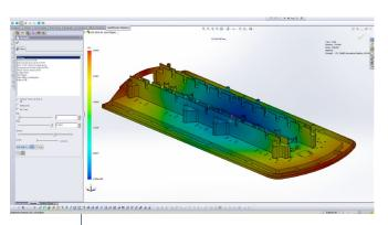
With SOLIDWORKS Plastics Professional tools, ECCO engineers can efficiently simulate mold filling, enabling them to optimize and speed up manufacturing.
