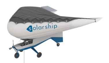
SOLIDWORKS Simulation capabilities are enabling Solar Ship to resolve one of its biggest technical challenges: understanding how to interface a large, rigid aluminum fuselage with a light, inflatable wing.
