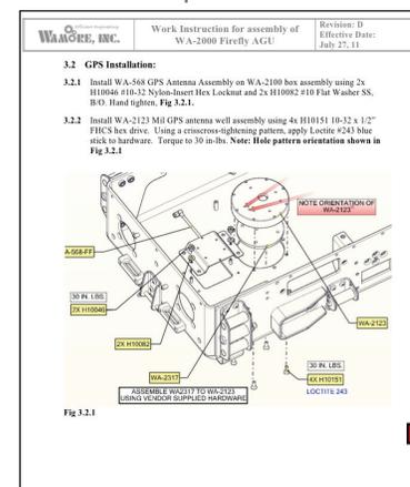
SolidWorks Composer software has enabled Wamore to replace assembly instructions that relied on unwieldy photographic images (top) with easy-to-understand, step-by-step instructions (bottom) that are developed in 85 percent less time.
