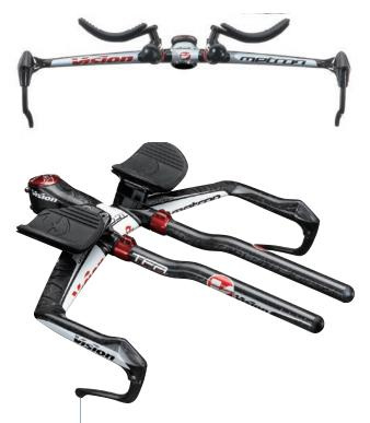
Full Speed Ahead used SOLIDWORKS Flow Simulation CFD analysis software to develop the fastest 3:1 aerobar, a specialized handlebar used by professional cyclists to support a more aerodynamic riding position.
