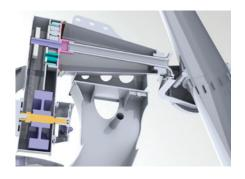
With SolidWorks Simulation software, ADES accurately predicted that its pendular wind turbine design would lower stress loads, extending a turbine tower's lifespan and lowering construction costs.
