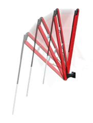
SolidWorks simulation tools allow JL Marine Systems to conduct motion and structural studies on the Power-Pole, reducing the number of prototypes required.
