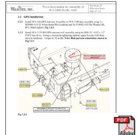
3D VIA Composer software has enabled Wamore to replace assembly instructions that relied on unwieldy photographic images (top) with easy-to-understand, step-by-step instructions (bottom) that are developed in 85 percent less time.
