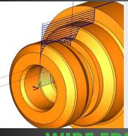
Lathe CAD-CAM makes it easy to set facing and OD/ID roughing, finishing, threading, and grooving 2 axis toolpaths on your CNC turning machine. Define custom tool holders, inserts and part holders for a realistic simulation experience to give you the peace of mind in knowing what will occur at your actual machine before ever cutting a chip.
