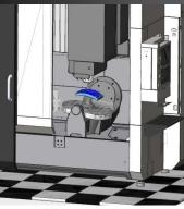
Visualize your machine in action within the CAM simulation window to test and confirm your toolpath programming on 2-5 axis CNC machines. This allows you to verify part fixtures are oriented correctly, machine movements are collision free, proper tool fixtures sizes are being used, and much more. The simulation play controls and move list allow you to easily isolate potential programming problems and quickly make the required adjustments.
