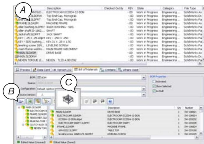
To make finding the required file even easier, SolidWorks Enterprise PDM employs both thumbnail and detailed 3D viewing capabilities, providing a visual way to find relevant models, drawings, and images.
