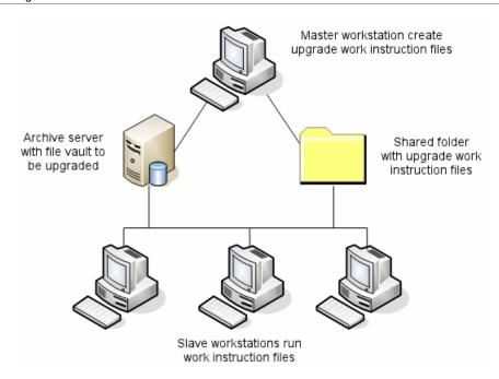
The work instruction files contain tree structures that reflect the parent-child relationships of the SolidWorks files. Both master and slave workstations can run additional work instruction files after they finish processing the first one. Although parts and subassemblies can be shared by other assemblies, each file is only upgraded once.
