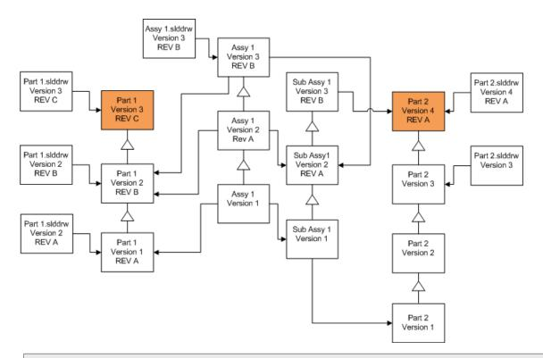
By default, part drawings are not upgraded. However, because drawings are parents to parts, a Broken reference warning screen lets you select to upgrade the drawings that reference the parts that are being upgraded.
