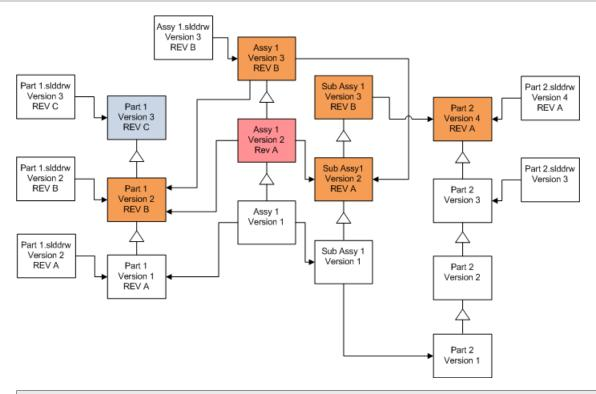
In a referenced version stream, the File Version Upgrade tool also upgrades the latest parts, as indicated by the blue boxes.
