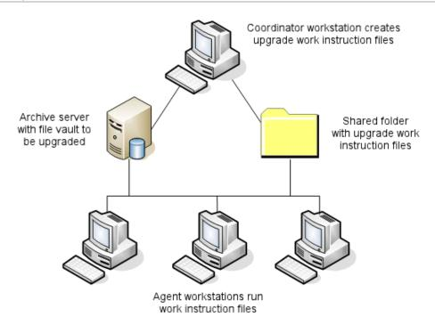
The work instruction files contain tree structures that reflect the parent-child relationships of the SOLIDWORKS files. Both coordinator and agent workstations can run additional work instruction files after they finish processing the first one. Although parts and subassemblies can be shared by other assemblies, each file is only upgraded once.
