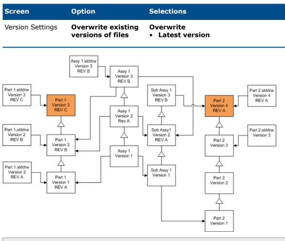
By default, part drawings are not upgraded. However, because drawings are parents to parts, a Broken reference warning screen lets you select to upgrade the drawings that reference the parts that are being upgraded.
