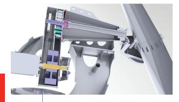
With SOLIDWORKS Simulation software, ADES accurately predicted that its pendular wind turbine design would lower stress loads, extending a turbine tower's lifespan and lowering construction costs.
