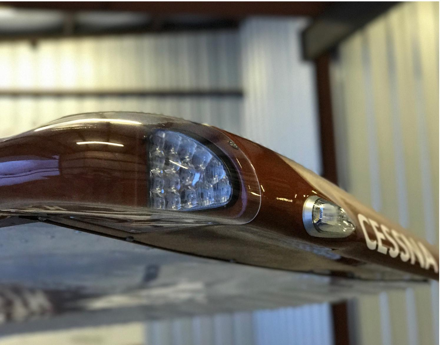
AeroLEDs leverages integrated SOLIDWORKS mechanical and PCB design solutions to support its rapid growth in the development of landing and navigational LED-based lighting systems. These systems are used on experimental, special-use, and military aircraft such as the lighting system installed on the wing of the Cessna™ aircraft shown here.
