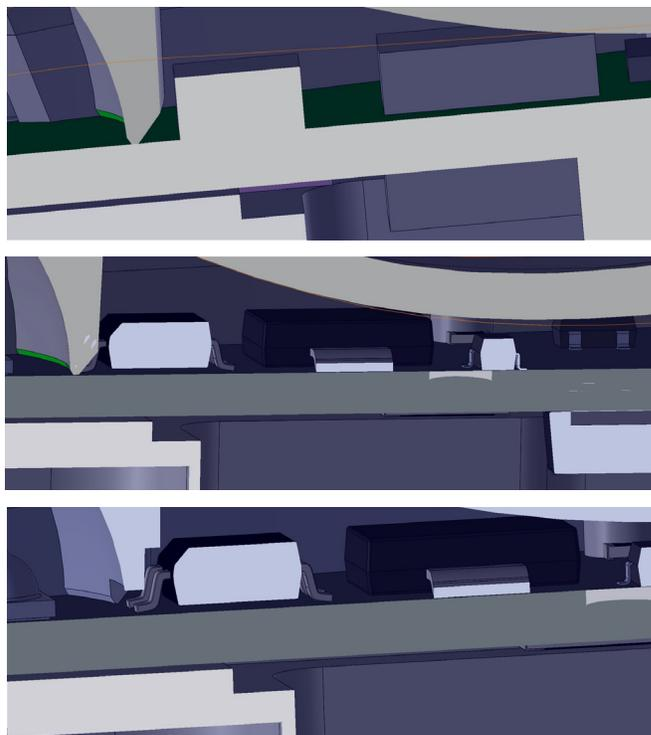
Before implementing integrated SOLIDWORKS PCB, AeroLEDs could not detect many interferences (top image) without going to the expense of ordering a prototype board. With SOLIDWORKS PCB software, interferences become obvious in SOLIDWORKS (middle image), where they can easily be resolved (bottom image) without incurring the time and cost of creating a prototype board.
