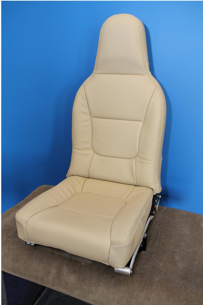
Using the combination of SOLIDWORKS Professional design and ExactFlat Design Studio 3D-to-2D flattening software, Aerosport has replaced its manual seat-pattern-making upholstery process with an automated digital approach, substantially reducing time-to-market and production costs.
