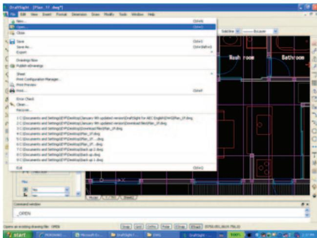
Edit the bearing mark of the reference source file "Site.dwg", and make the changes made in this source file appear on the current drawing. Leave the current drawing as it is, and open "Site.dwg".
