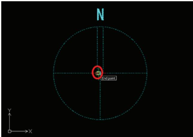
④ To “Specify pivot point”, specify the point that would be the center of rotation.
