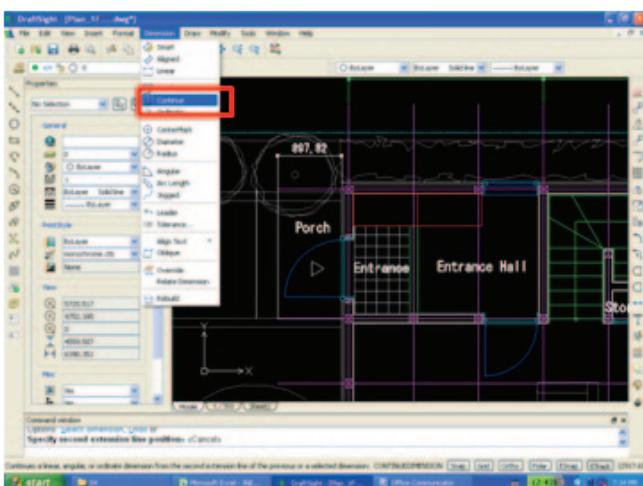
Enter the dimension of the elevated level of the porch. Here, we will use the Continue command because we are going to enter another dimension in series.
