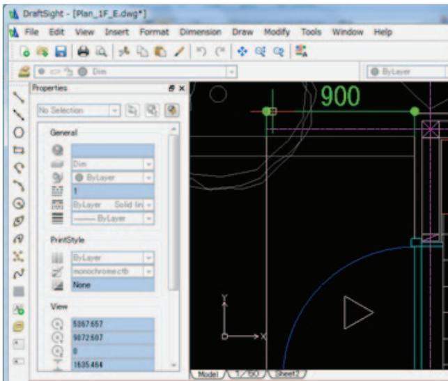
⑤ To Specify dimension line position>>move the cursor upward and click any desirable position randomly.
