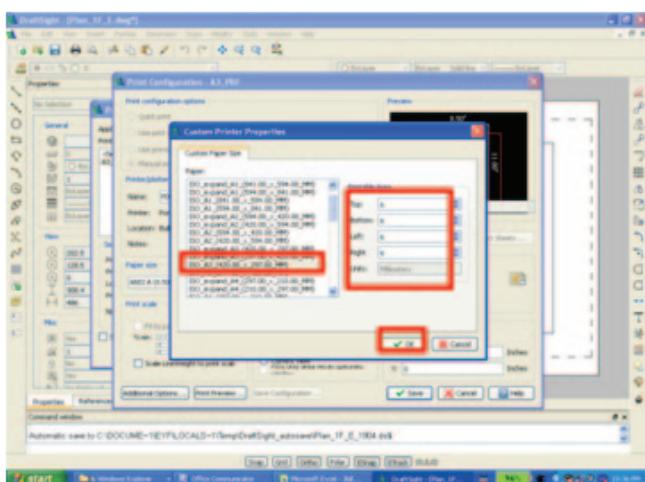
⑦ "Custom Printer Properties" dialog window appears. For the type of "Paper", select "ISO\_A3\_(420.00\_X\_297.00\_MM)". Set "6" for all the margins (Upper / Lower / Left / Right) of the "Printable area". Click "OK" after completing the above setting.
