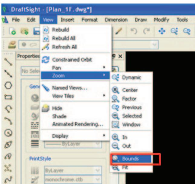
Use the “Boundary zoom” command to display the entire drawing. By using the “Bounds” command, you can make all the entities of the drawing appear on the drawing workspace.
