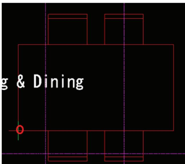
⑦ To "Specify insertion base point»", place the cursor in the lower left corner of the table, click when the endpoint snap appears.
