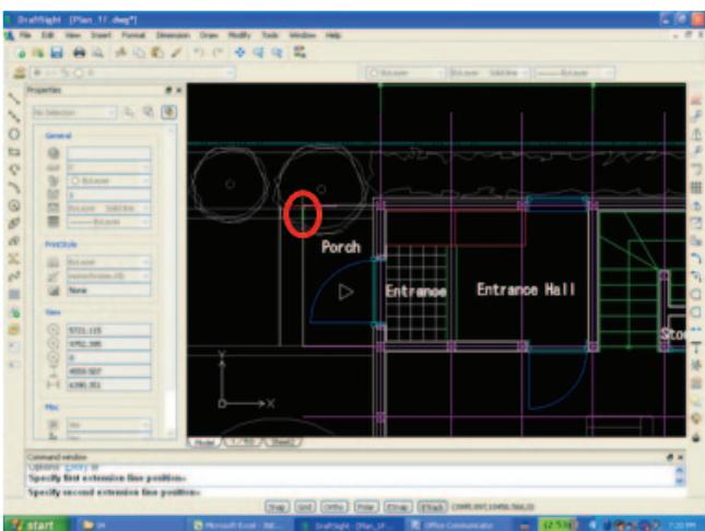
④ To be capitalized second extension line position>>place the cursor to the edge point of the line that has been offset in the beginning, and click when the endpoint snap appears.
