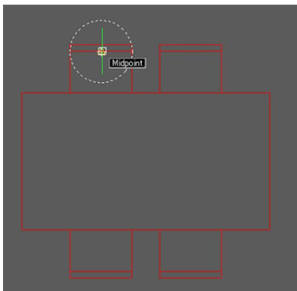
⑩ To "Specify the strating point»", specify the midpoint that is at the same position as the point specified at the center of the circle by using the midpoint snap method.
