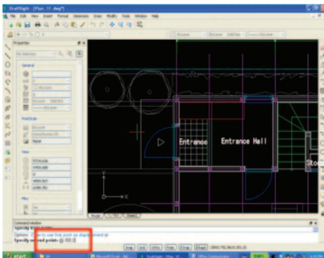
⑤ To "Specify second point", enter the coordinate values "@-300,0" by using the keyboard, and press "Enter". Then a duplicate line will appear at point -300 in X direction and point 0 in Y direction from the starting point.
