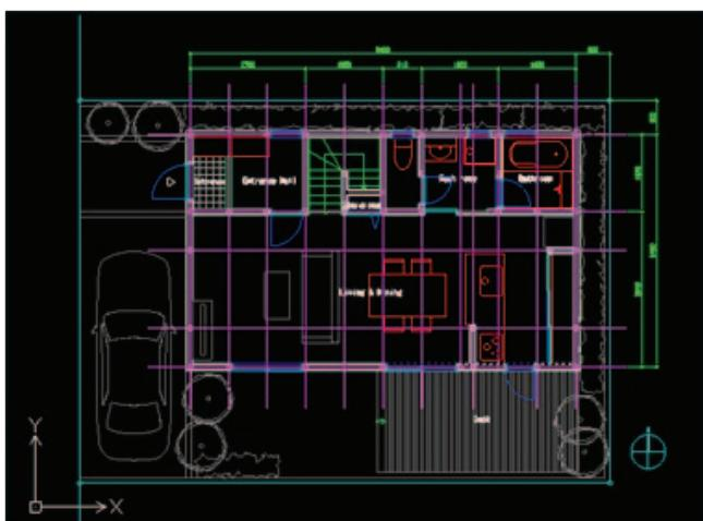
Then the Layers "External Element" will be switched to hide the mode. As a result, the automobile as well as all other objects belonging to the "Exterior" group will no longer appear on the displayed drawing.
