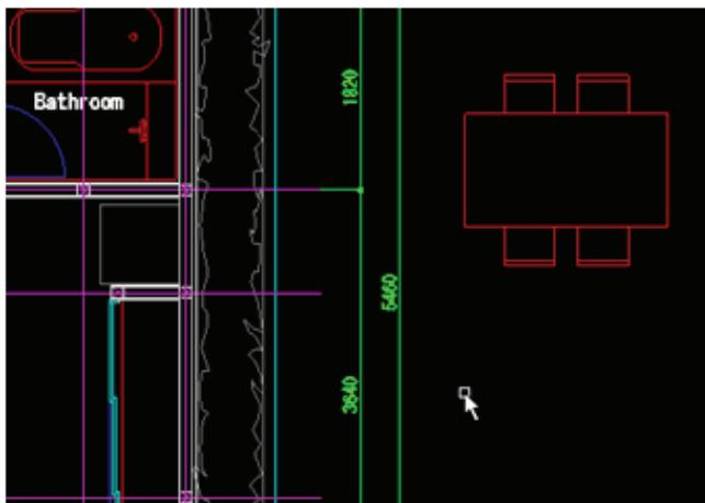
④ The “Dining Set” block will appear on the cursor. To “Specify destination>> select a desirable point randomly somewhere in the open space on the right side of the screen, and click to insert the block.
