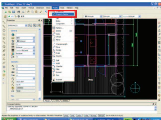
Now, we need to do the same for the Layer where the chairs are sorted. This time, rather than following the same procedure taken to change the name of the Layer where the table is sorted, we will try another method, which is to copy the Layer property of the table.
