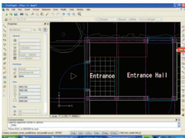
Use the Offset Command to draw the different levels of the porch. Draw a porch that is 900 in width and 300 in elevated level.
