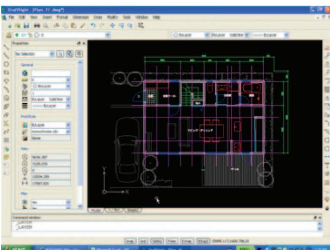
The unnecessary data will not be displayed, and the referenced drawing of the premise will appear clearly.
