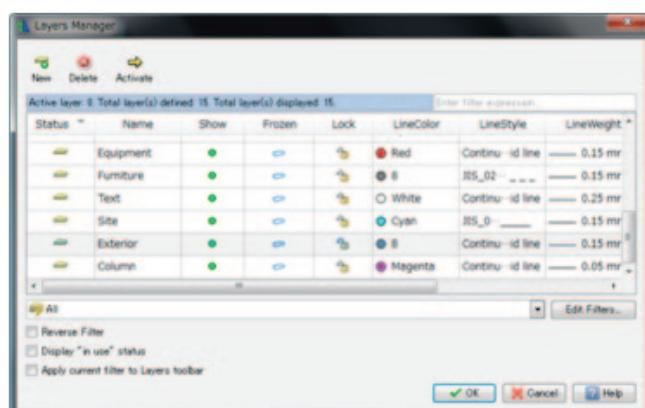
② In the same procedure explained earlier, display the Layer Manager, change the color of the circle in the row "Exterior " under the "Show" column to grey, and click the OK button to close the Layer Manager.
