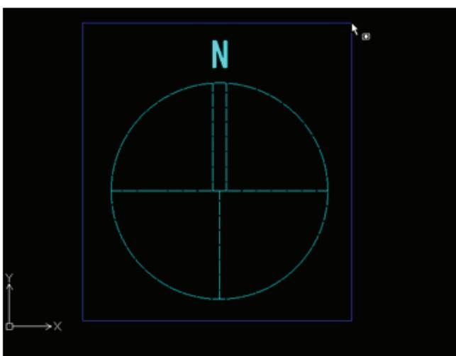
To "Specify entities»", click the lower left point of the rectangle surrounding the bearing mark to select it to rotated the bearing mark and display it on the window. A blue rectangle will appear as a temporary rectangle. Click the upper right point of this rectangle. Press "Enter" to complete the selection of the graphics.
