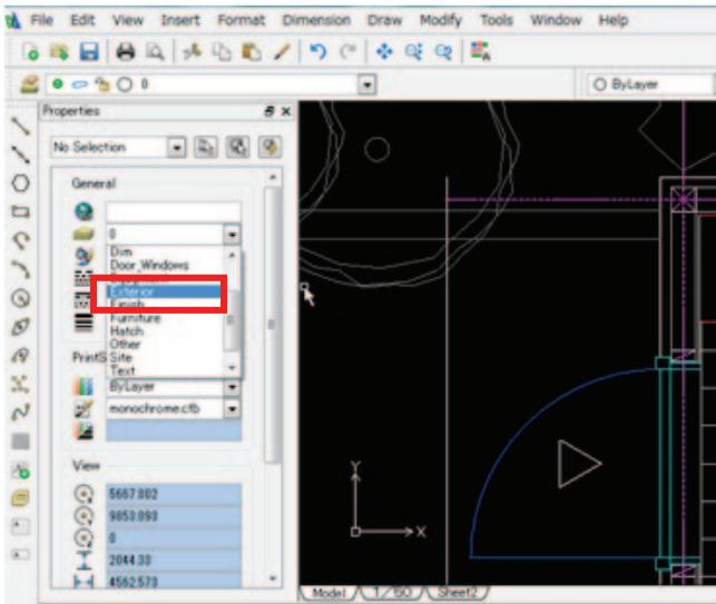
② From the pull-down menu that lists the Layer items located in the Property Pallet on the left, select "Exterior" to change the Layer for the offset line to this item.
