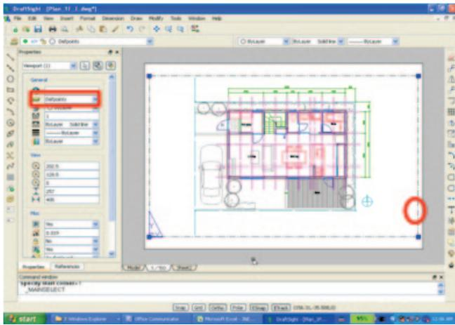
By using the ViewPort that has been adjusted to be as large as the printing area, create the view for displaying the model.
