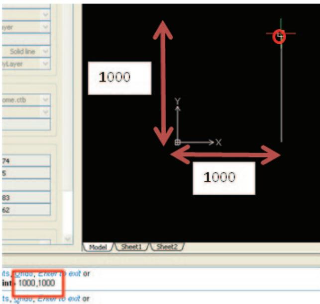
③ Next, specify “1000,1000” as the next point and press “Enter”. Then a line segment will be drawn to point 1000 in X direction and point 1000 in Y direction from the point of origin.
