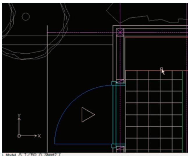
② For Specify cutting edges>> click the grey line located on the lower side of the external element area. Press "Enter" to end the operation of selecting the cutting edges.
