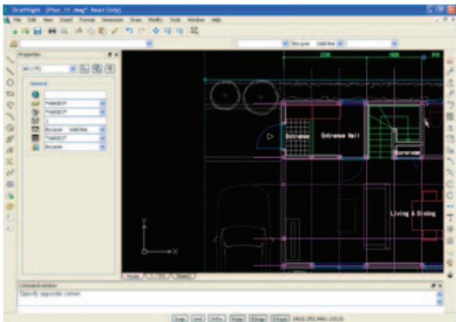
The drawing zooms in from the center of where the mouse pointer is pointing.
