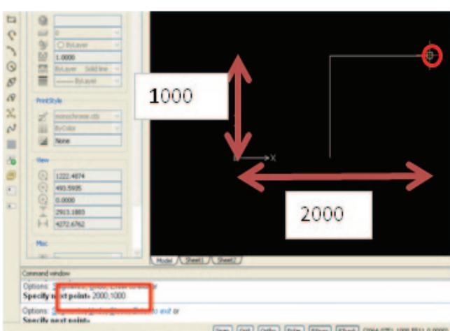
④ Next, specify “2000,1000” as the next point and press “Enter”. Then a line segment will be drawn to point 2000 in X direction and point 1000 in Y direction from the point of origin.
