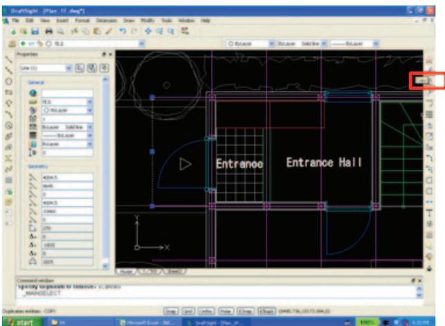
Copy the offset line to the position 300mm left of this line to represent the additional level of the porch.
