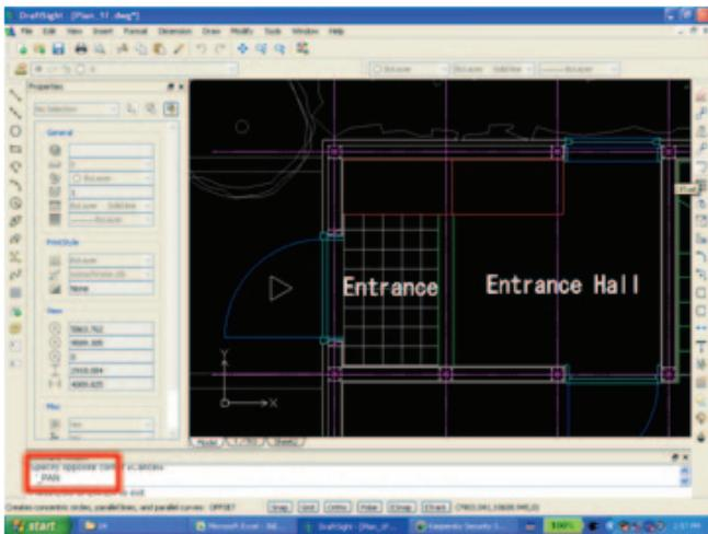
③ You now want to draw a line that ends at a position 900mm away from the outer wall surface. Enter "900" by using the keyboard and press "Enter".
