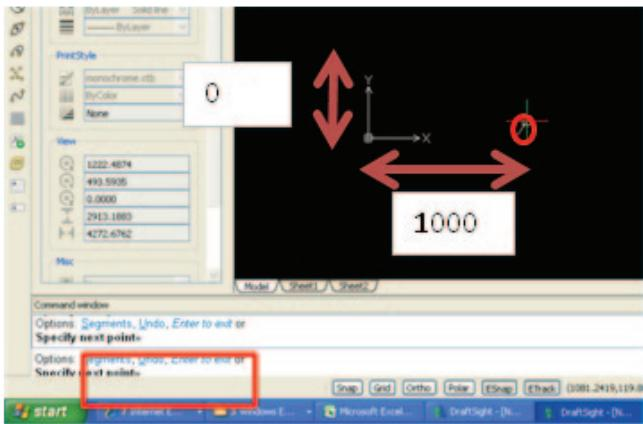
② As the command for specifying the starting point, enter “1000,0” as the absolute coordinates by using the keyboard and press “Enter”. Then a line will be drawn to point, 1000 in X direction and point 0 in Y direction from the point of origin (0,0).
