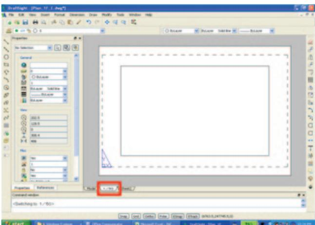
Configure the sheet for printing by specifying the printer and paper size using the Printing Configuration functionality.
