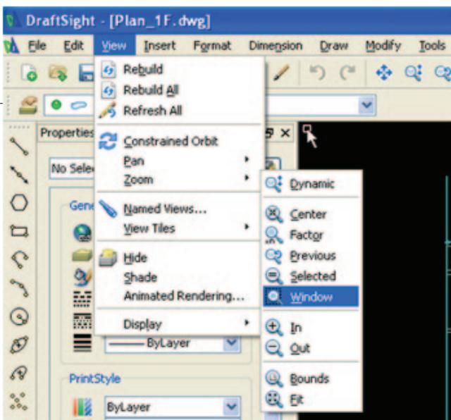
Window zoom functionality is used to enlarge the specific area of the drawing by surrounding the desired area with the boundary of the window and displaying the area captured within the boundary fully on the window.
