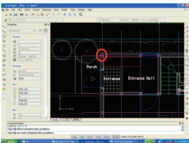
③ To be capitalized first extension line position>>place the cursor to the point where the grey line of the external element and the outer wall line intersect, and click when the endpoint snap appears.
