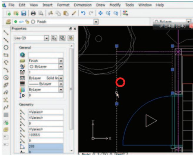
The offset line currently belongs to the Offset Source Property, and is sorted in the Layer called "Finish". We will change the Layer for the Offset Line to "Exterior".
