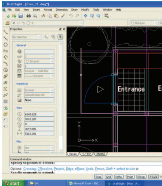
⑤ Press "Enter" to end the operation of extending the specified line.
