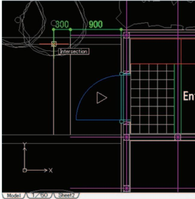
⑦ To specify second extension line position>>place the cursor to the edge point of the elevated level that has been copied, and click when the endpoint snap appears.
