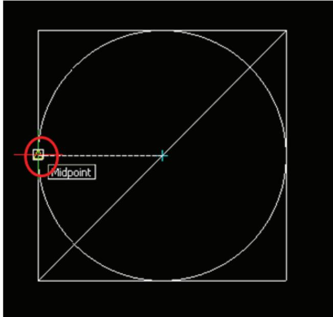
⑤ Move the cursor to the middle of the left side of the square. At this point, only the Midpoint Snap can be used. Place the cursor at the position where the Midpoint Snap appears, and click to specify the midpoint of the left side.
