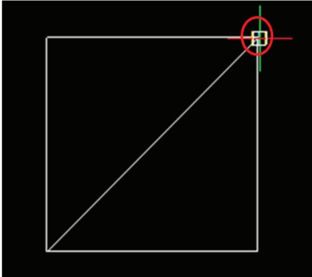
④ Move the cursor to the direction of the diagonal line, and place it on the upper right vertex of the square. Just like in the previous step, place the cursor at the position where the Endpoint Snap appears, and then click to specify the end point of the line segment.
