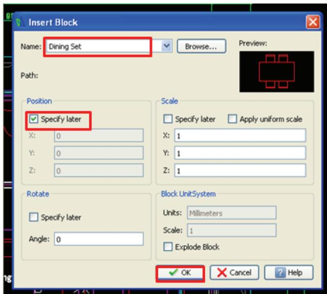
③ "Insert Block" dialog box will appear. Select "Dining Set" from the pull-down list opened at the Name field. Place a check next to "Specify later" under the Position column. Then click "OK".
