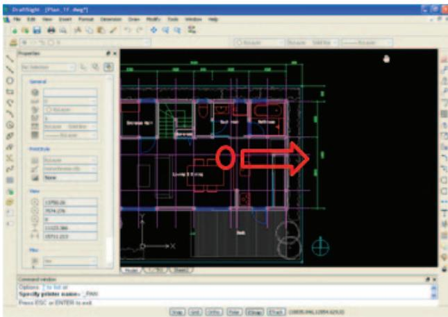
③ Press the mouse wheel button again, and while pressing it, drag the drawing to the right and then release the button.
