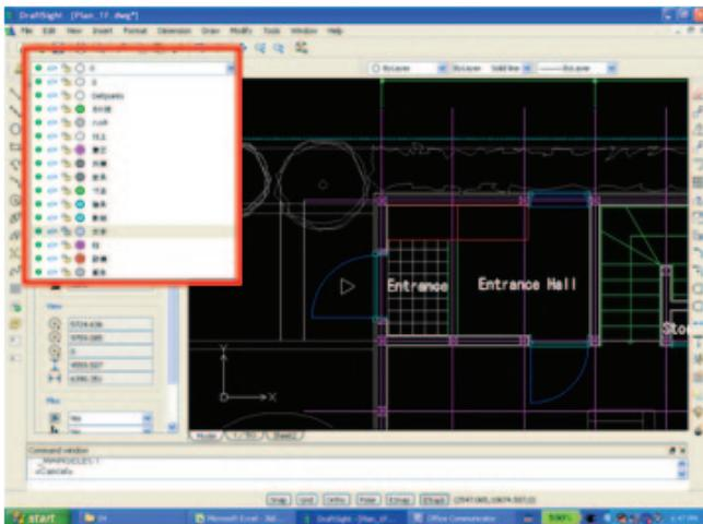
Enter the text "Porch" anywhere close to the line that has just been added. Since we are going to enter text, we need to change the active layer to "Text".
