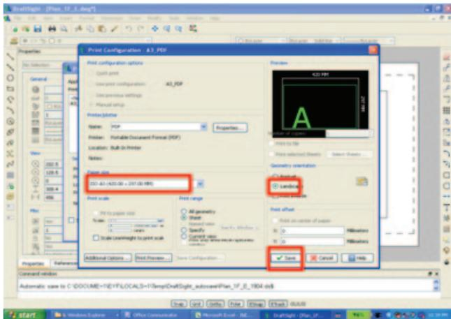
⑧ On the “Printing Configuration” dialog window, select “ISO\_A3\_(420.00\_X\_297.00\_MM)” as the “Paper size”. Select the radio button next to “Horizontal” for the “Geometry orientation”. Then select “Save”.
