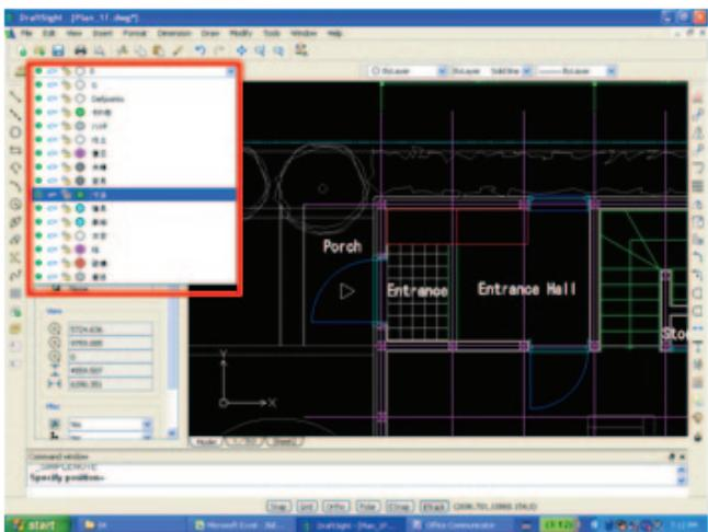
Now, let's enter the dimensions that represent the width and the elevated level of the porch. Since we are going to enter the dimensions, we need to change the active Layer to "Dimensions".
