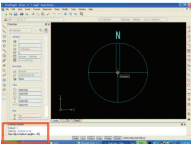
⑤ To “Specify rotation angle”, enter “-45” with the keyboard and press “Enter”.
