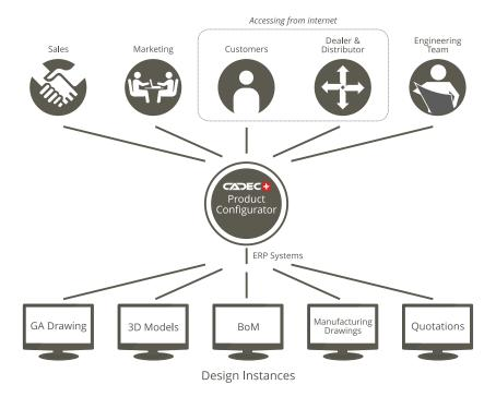
CADEC+ Empower accesses enquiries data from RDBMS and stores design output data in an RDBMS. The enquiry database can be updated by ERP enquiries and the design output data can be accessed by ERP for BOM, Cost sheet, Quotation, Drawings.
