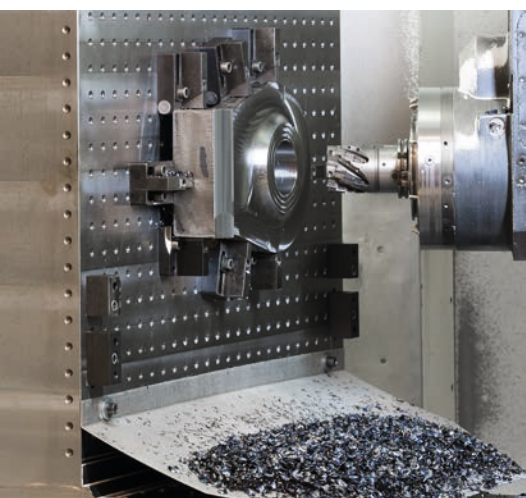
The iMachining technology reduces the strain on the spindle, guides, and mount. In heavy machining, this results in reduced machine wear and increased service life.
