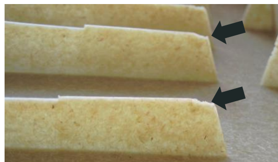
Figure 9: Accurate simulation of filling behavior for a fiber-reinforced material helps identify filling issues
