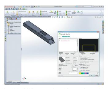
Lantek Flex3d Addins recognises and imports tube parts from standard formats such as round, rectangular and square. It is also possible to import combined structures of sheet and tube
