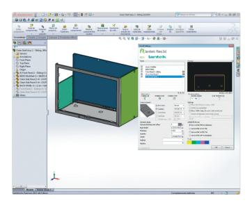
A preview of each flat pattern is shown following part unfolding prior to its final transfer to the Lantek management system.
