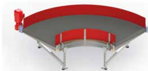
3D view of a curved belt conveyor created with Tacton Design Automation in Solidworks®.
