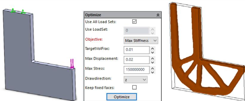
Figure 12: ParetoWorks is constraint driven.
