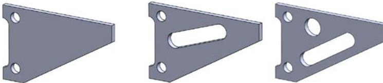
Figure 2: Finding light-weight designs however is a trial-and-error process.
