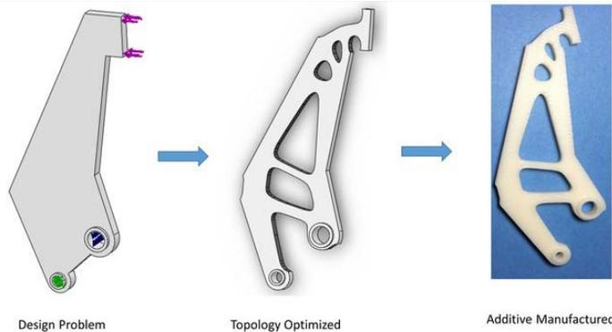
The output from topology optimization can be directly 3D printed, or used as a concept in traditional CAD.
