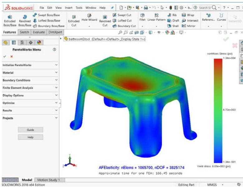
Figure 11: ParetoWorks has a built-in FEA solver.
