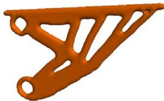
Figure 3: An optimal topology for the problem in Figure 1a.
