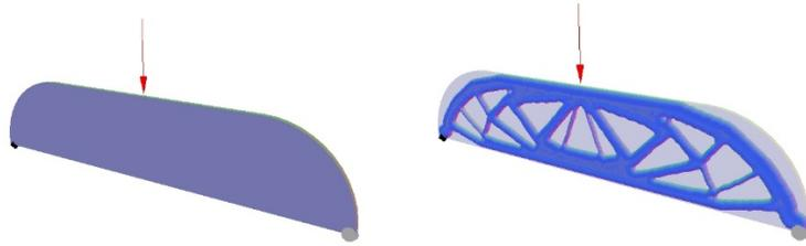
Figure 6: (a) A bridge-design problem, and (b) topology optimized design.
