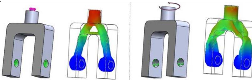
Figure 7: Topology optimized design under (a) tensile loading, and (b) torsional loading
