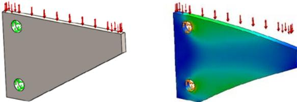
Figure 1: (a) A structural problem: reduce the weight by 50%. (b) FEA provides hints where to remove material
