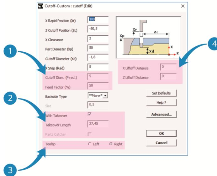
1 The new settings “*Cutoff Diameter (F-reduced)*” and “*Feed Factor*” allow performing the final stage of the cutoff process using a reduced feedrate.
