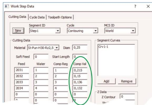
The “*Comp-Val*” section where the offset for each pass is defined
